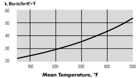
Apparent thermal conductivity curve determined in accordance with ASTM Practice C 1045 with data obtained by ASTM Test Method C 335. Values are nominal, subject to normal testing and manufacturing tolerances.
